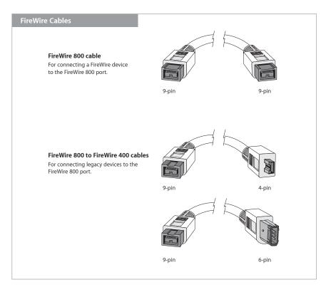
FireWire 400 devices use a 6-pin or 4-pin connector; FireWire 800 devices use a 9-pin connector. The FireWire 400 ports on Apple systems have 6 pins, while the FireWire 800 ports have 9 pins. Existing FireWire 400 devices can be plugged into either type of port, although in some cases an adapter cable (4-pin to 6-pin, 6-pin to 9-pin, and so on) is required. FireWire 800 devices can achieve FireWire 800 speeds only on the FireWire 800 port.
